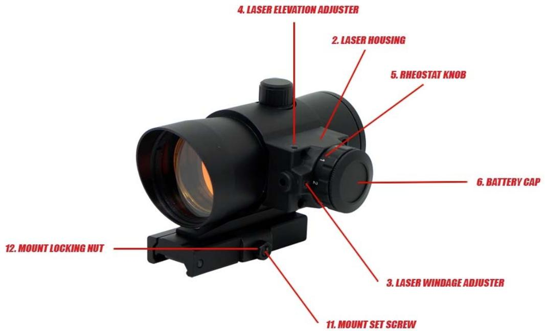
1. Begin by loosening the *Mount Locking Nut* (12) on the left side of the mount. To perform this action, be sure that the *Quick Release Lever* (10) is in the closed position pointing towards the eyepiece. Using a wrench, turn the *Mount Locking Nut* (12) counter-clockwise.
