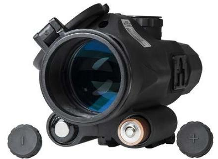
Remove the (+) Battery Cap (right side) by turning it Counter-Clockwise (⤿) and Remove the old battery and dispose of it properly. Replace it with a New 1.5V AA Battery, with the positive (+) side facing outward. Reinstall the Battery Cap by twisting it Clockwise (⤵) until snug. You may have to push the cap down towards the threads, pushing against the spring inside the (+) battery compartment, for the cap to engage the threads.
